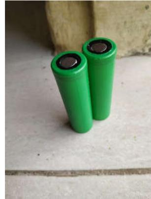
Gambar 5. Baterai lithium ion 18650
